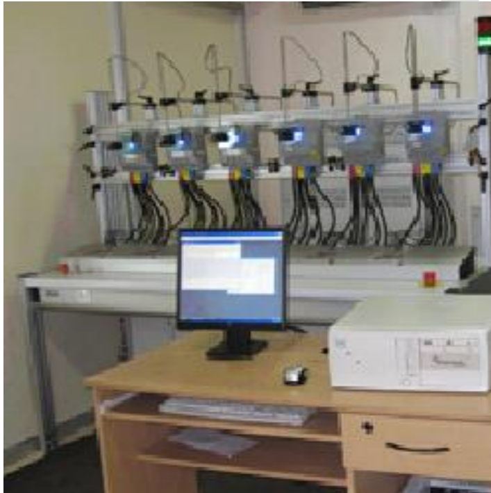
Energy Meter Test Bench
