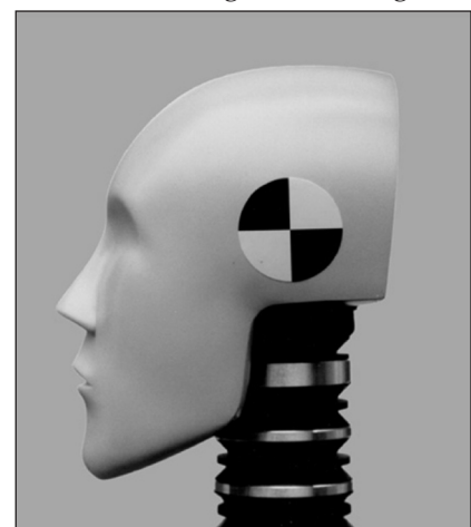
Figure 2. Yellow-black color pattern target on a dummy for car crash test
