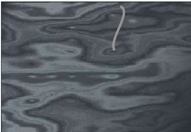
Fig 6: A needle-like tin whisker.
