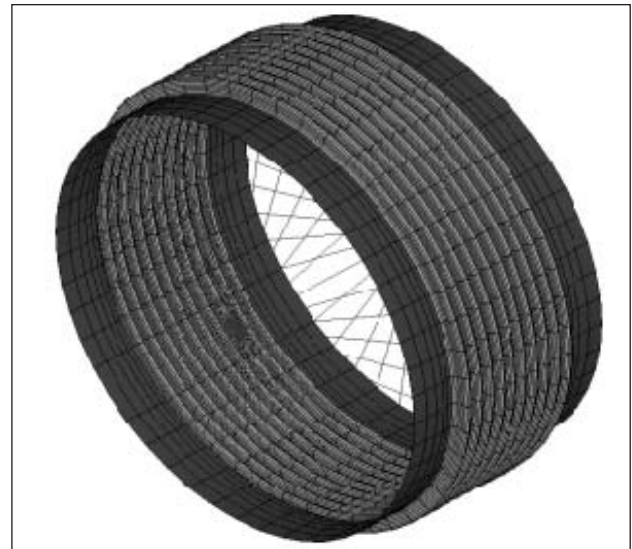
Fig.6: Finite element model of expansion bellow at the RCB penetration of PFBR
