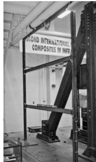
Figure 2. Experimental Verification of a Scaled 2D frame
